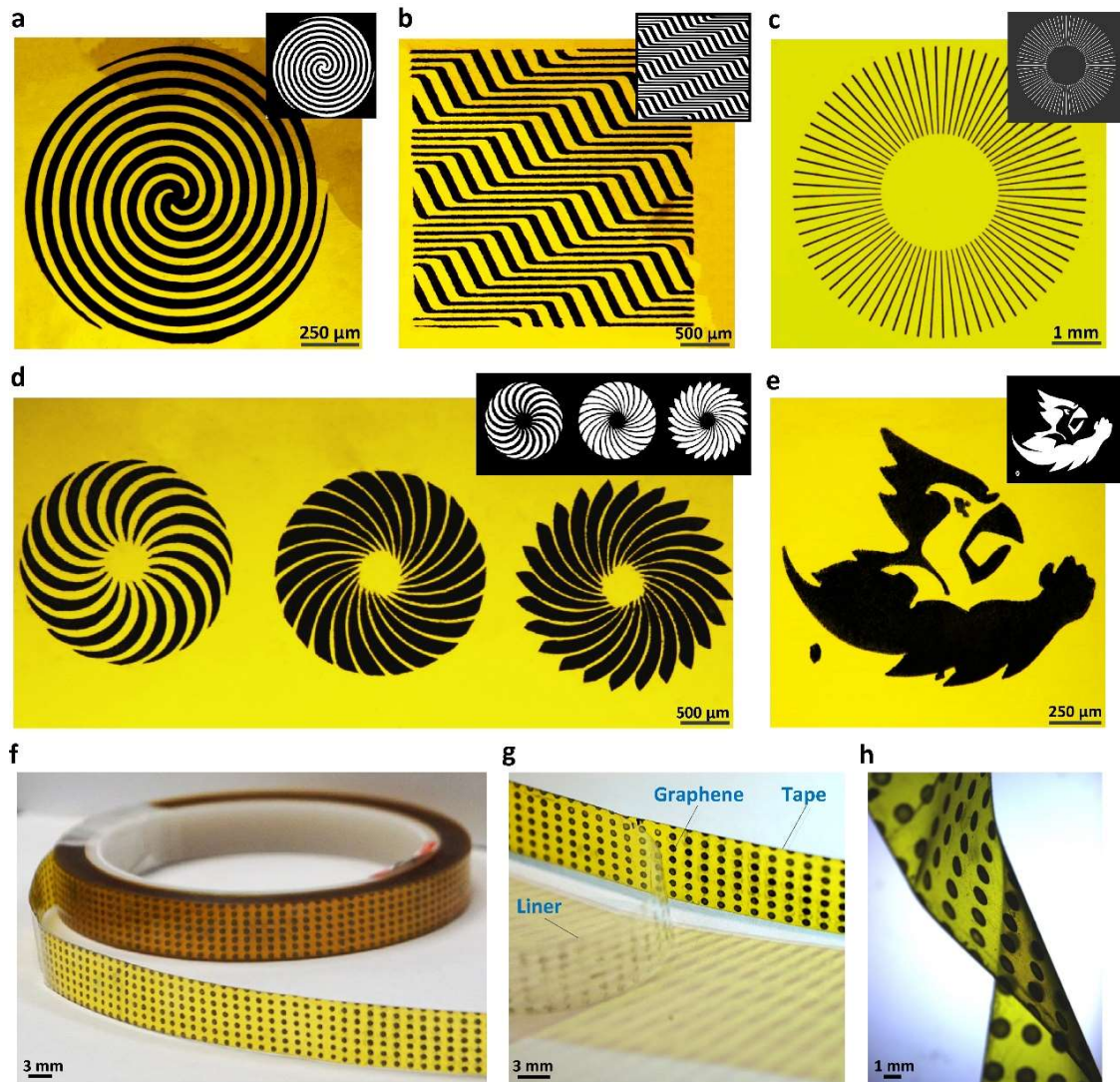
Figure 2.2 (a)–(e) Versatile graphene patterns formed on the polyimide tape using the proposed method. (f)–(h) Formation of graphene patterns on the relatively large polyimide tape roll with liner. The transferred graphene patterns are protected by a non-sticky liner.
